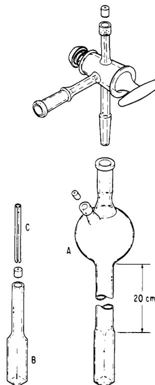
**Figure 14.** Tonometers for spectroscopic and kinetic studies. B is a 6-mL liquid phase tonometer of variable size and A is a 130-mL gas-liquid tonometer for vacuum line methods.
